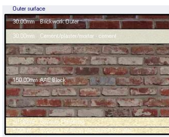
Figure 4. Baseline exterior wall materials.
